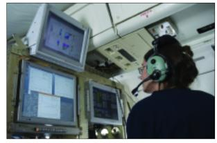
Susan Kool monitors data from the Lidar Atmospheric Sensing Experiment (LASE) instrument on board a NASA DC-8 aircraft flying through a Saharan dust storm over the Atlantic. Researchers hope to use these data to track interactions between the dust and tropical storms and to better understand Atlantic hurricane development. (Courtesy NAMMA team)
