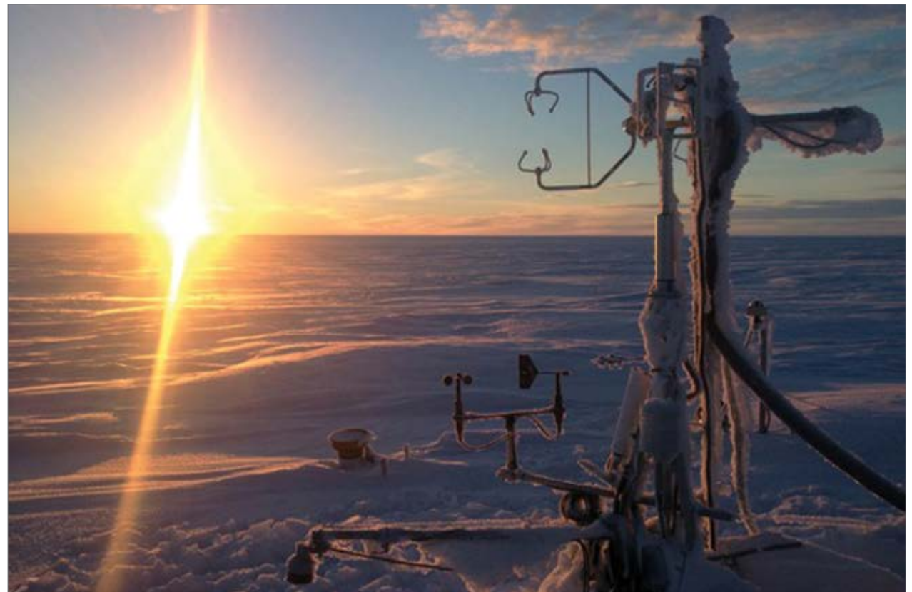
Frost clings to an eddy covariance tower in Barrow, Alaska. The sensors measure methane emissions year round and are equipped with deicers to prevent them from malfunctioning in the Arctic’s frigid temperatures. The tower also measures other meteorological variables, including air temperature, humidity, soil temperature, and soil moisture. (Courtesy S. Losacco)
