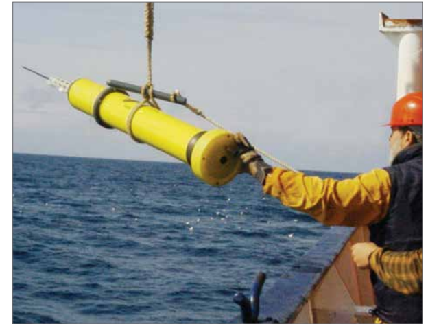
Researchers deploy an Argo float, a submersible instrument that records ocean temperatures and other data up to 2,000 meters (1.24 miles) deep. (Courtesy Argo Program)
