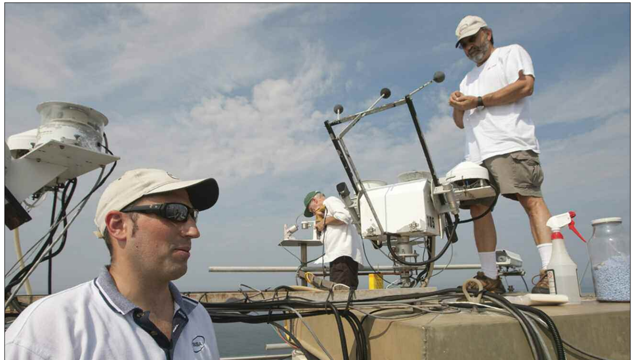
At the CERES Ocean Validation Experiment (COVE) lighthouse site, Bryan Fabbri (left), Fred Denn (middle), and Bob Arduini check on several instruments on top of the lighthouse tower. The instruments help validate satellites that measure clouds and Earth’s energy budget. (Courtesy S. Smith, NASA Langley Research Center)
