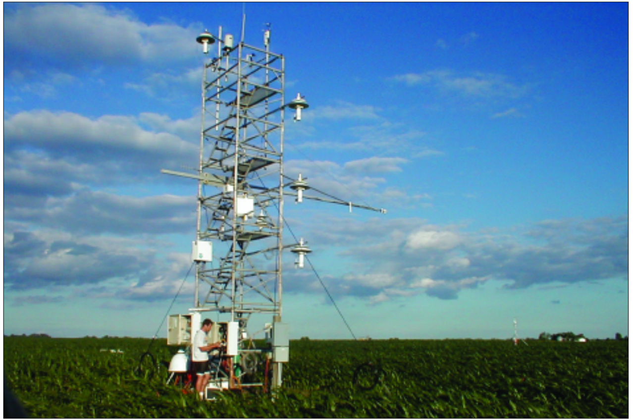
This FLUXNET tower is one of many worldwide that scientists have erected to constantly monitor landscape health and productivity. They hope to better understand the energy exchanges that are essential to the lifecycles of vegetation. (Courtesy FLUXNET)
