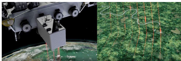
Left: This graphic shows the GEDI instrument's three lasers, which are split into eight tracks. Each laser fires 242 times per second and illuminates a 25-meter footprint on the surface within which four surface parameters — surface topography, canopy height metrics, canopy cover metrics, and vertical structure metrics—are calculated. Right: This graphic shows the eight tracks sampling the Earth's surface with between-track spacing of about 600 meters (1,969 feet) and a total width of 4.2 kilometers (about 2.6 miles) across all eight tracks. (Credit: NASA's Goddard Space Flight Center)
