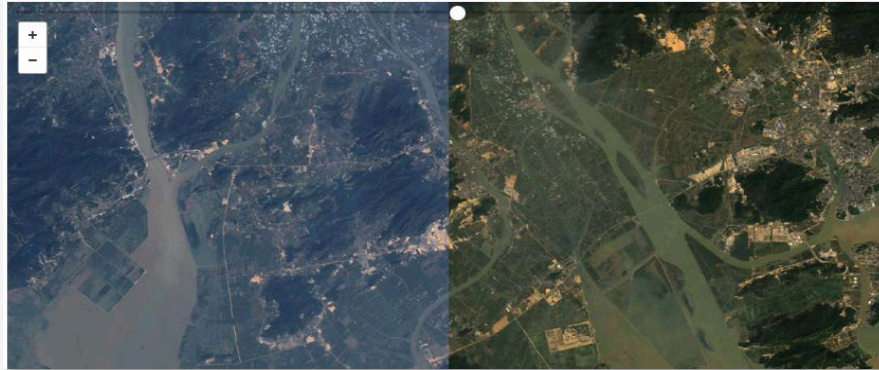
Example of the unprocessed Landsat image (left) and the LEDAPS processed Landsat image (right)
