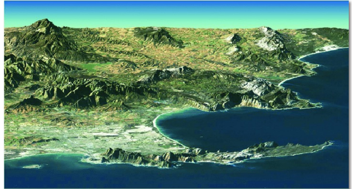
Landsat data to texture-map the surface created using the SRTM elevation data. Image Credit: NASA
