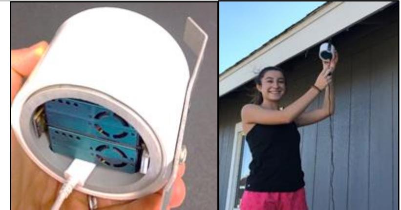
Top: AirNow Fire and Smoke Map showing sensor locations each displaying the current NowCast AQI (accessed 7/15/25). Bottom left: PurpleAir PA-II-SD outdoor sensor. Bottom Right: Intern installing a sensor at a Nez Perce library.
