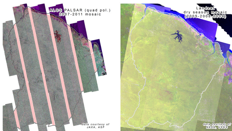
Figure 8.5 Contrast between polarimetric ALOS PALSAR data (left) and Landsat multispectral imagery (right) of French Guiana (Cherrington 2016).
