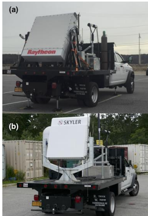
Figure 2: (a) SKYLER-I and (b) SKYLER-II on the SBU weather mobile platform. (Image source: Radar Science SKYLER webpage )
