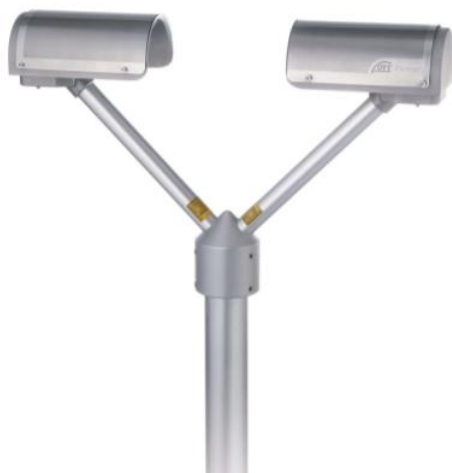
Figure 2: OTT Parsivel Disdrometer (Image source: OTT Parsivel document )
