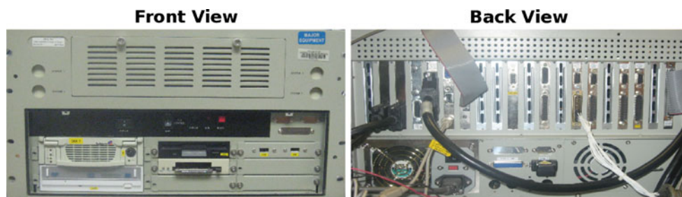
Fig. 1 Science Engineering Associates, Inc. model M300 Data Acquisition System used for aircraft field projects at the University of North Dakota
