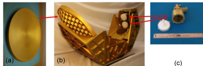
Fig. 5. HIWRAP antenna (a) main reflector. (b) Antenna assembly on the flight frame. (c) One of the dual-frequency feeds.
