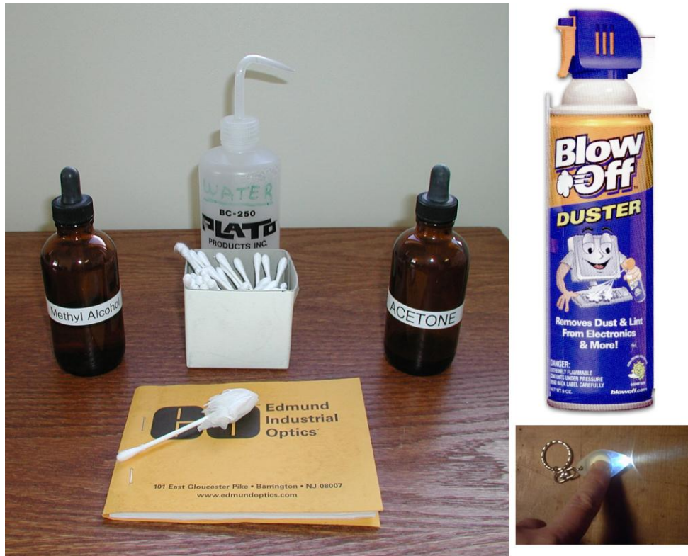
Figure 8.1.1. Items required for cleaning
