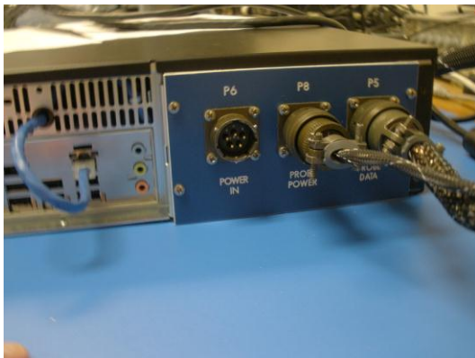
Figure 2.2.3 Probe Data cable connection
