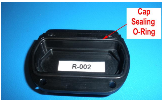
Figure 8.2.5. Inspect the Cap Sealing O-Ring
