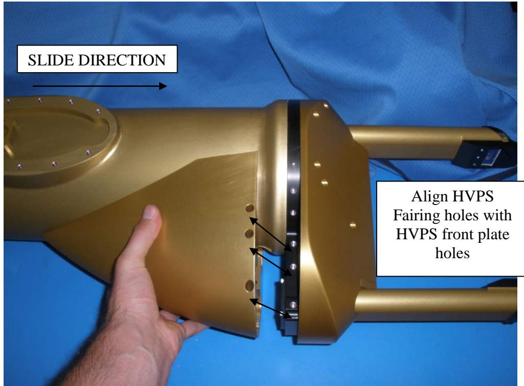
Figure A3. Installing HVPS Fairing
