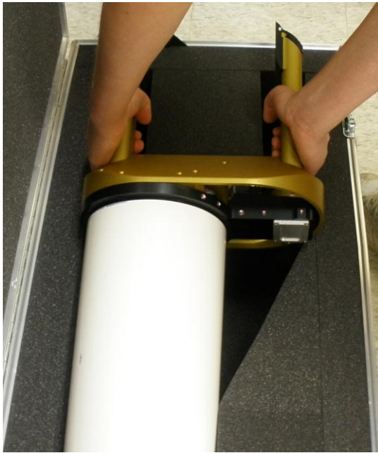
Figure 2.0.1 Correct probe handling
