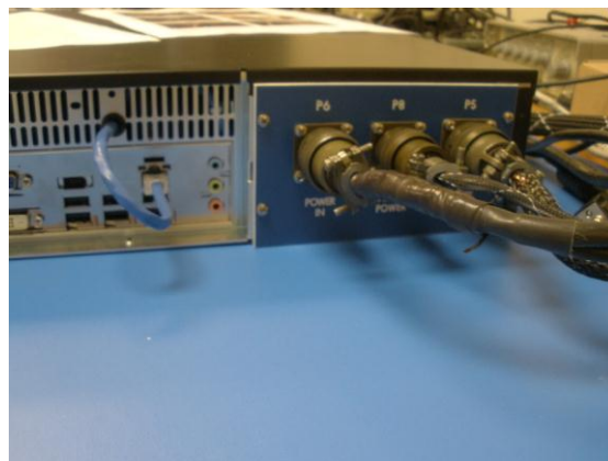
Figure 2.2.5 Data rack power cable connection
