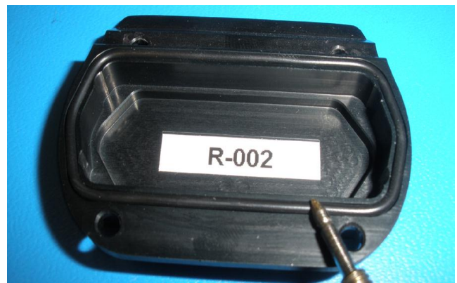
Figure 8.2.6 Push back the O Ring with thin, blunt object
