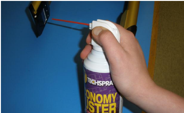
Figure 8.1.2 Using compressed air to blow off particles from windows
