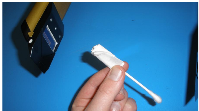
Figure 8.1.3 Optical quality cleaning tissue to clean windows
