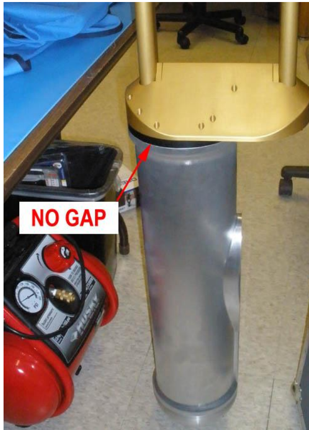
Figure 7.1. Probe properly installed in PMS Can
