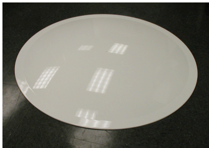
Fig. 6. WB-57 dual-frequency Ku- Ka-band radome
