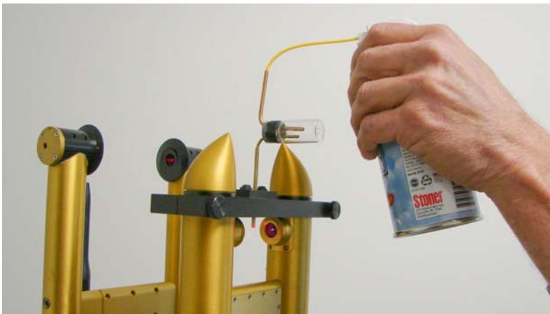
Figure 14: Releasing Glass Beads into the CDP. Note this picture is of a CDP attached to a CCP; operation is the same for stand-alone CDPs.
