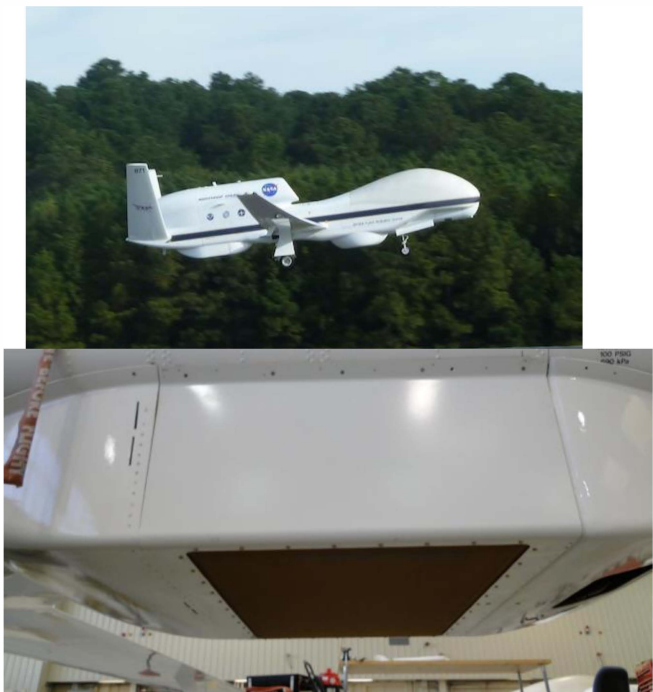
Figure 5. The NASA Global Hawk (above) and a closeup of its HIRAD installation (below).
