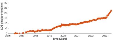
This OPERA DISP time series shows line-of-sight (LOS) surface displacement for the Portuguese Bend landslide, Palos Verdes, CA between 2016-2023. DISP products are derived from InSAR observations and will provide data for enhanced surface displacement analysis.
