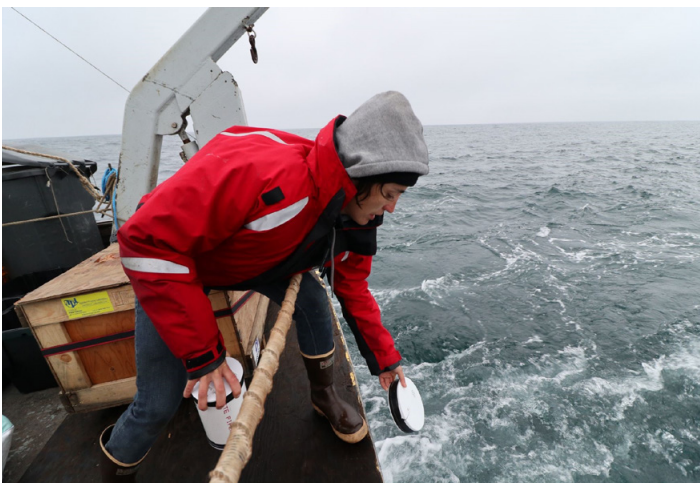
Dr. Kyla Drushka deploys ocean drifters to measure ocean currents at the sea surface. Drushka and her colleagues used these and other devices during a 2018 campaign she co-led off of the California coast near Monterey/San Francisco. Credit: Peter Gaube
