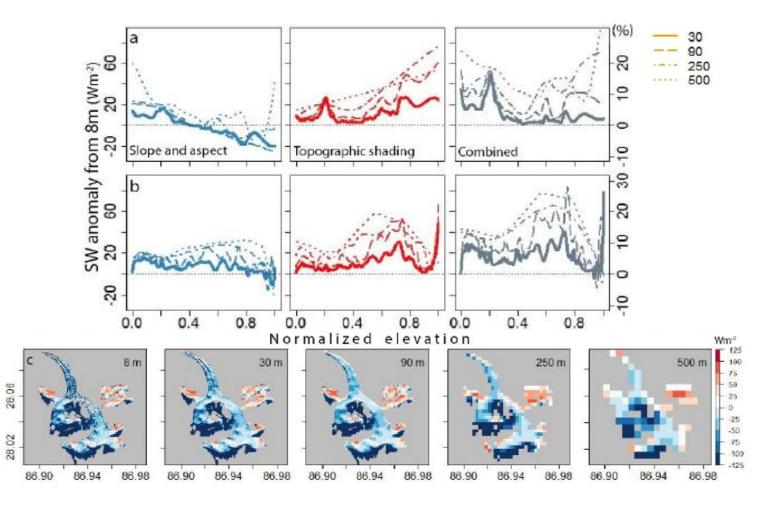
The Shortwave anomaly is the difference between the change in irradiance determined at each coarse DEM resolution relative to the change in irradiance calculated with the 8-m HIMAT DEM. The anomaly is shown at 30-, 90-, 250-, and 500-m resolutions for the East Rongbuk Glacier (a, top panels) and the Lumsamba Glacier (b, middle panels) on March 21. Panel (c) shows the combined change in irradiance due to all terrain attributes on this day at each down sampled resolution for East Rongbuk Glacier.
