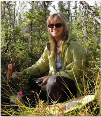
Dr. Laura Bourgeau-Chavez using a handheld water content reflectometer to measure soil moisture at a field site in Delta Junction, Alaska. Image courtesy of Dr. Bourgeau-Chavez.
