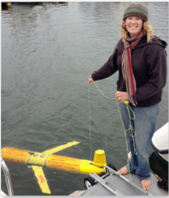
Dr. Bridget Seegers conducting a ballast check on a glider (yellow, airplane-looking object in water) during a West Coast project to better understand the initiation of harmful algal blooms (HABs).
